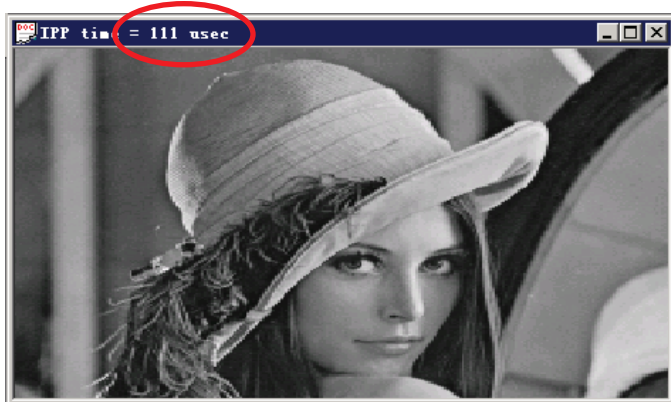
Figure 6. In this image-resizing example (from 256 x 256 bits to 460 x 332 bits), the Intel® IPP-powered application ran in 111 msec vs. 338 msec for compiled C++ code (system configuration: Intel® Xeon®, 2.9 GHz, 2 processors, 4 cores/processor, 2 threads/processor)
